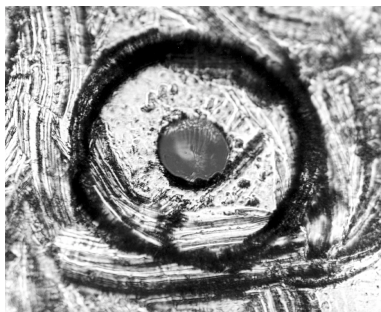
Figure 1-15. Damage from improper cleaning.
